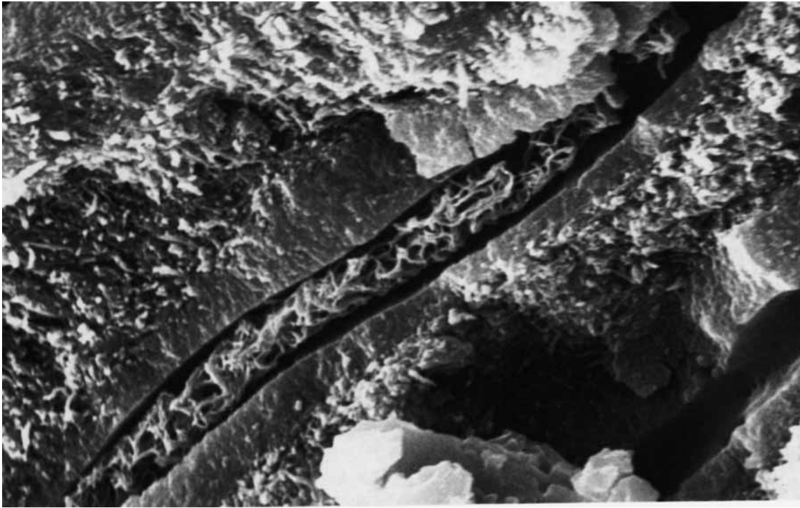
Figure 9(a) SEM photomicrograph of a tooth channel blocked by the poly(acrylic acid)- \text{FeCl}_3 (2 : 1) gel (G-IC). Scale bar 1 \mu\text{m} (photograph by E. Adamczak and J. F. Rabek).
